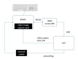
Fig. 4. KORAT Capture/Replay architecture with keyboard.
