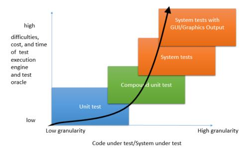
Fig. 1. The technical difficulties of test execution engine and test oracles as the granularity of code under test grows.
