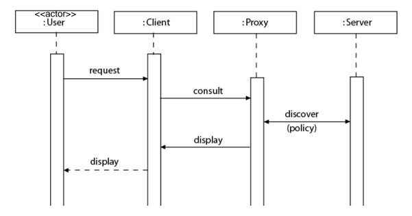
Figure 2: Sequence diagram for performing an interaction through a privacy-aware client.
