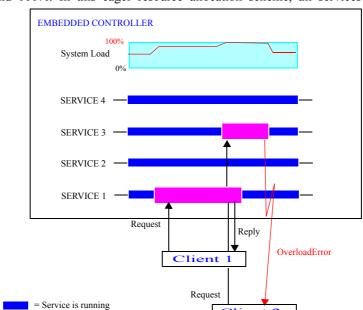
CPU load of the embedded controller that falls into the range between 0% and 100%. In this eager resource allocation scheme, all services are
