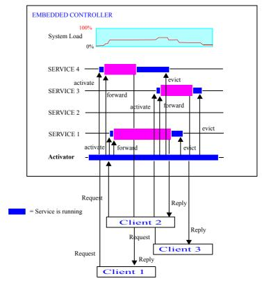
Example section, only a small number of clients could access the system simultaneously since scarce system resources were devoted to running unused services. In the refactored implementation, however, a larger number of clients can access the same (or different) services simultaneously without incurring overload. Even three clients concurrently accessing the embedded controller do not incur more than 50% CPU load, so the overload threshold will not be reached.
