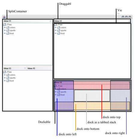
Figure 3. Basic elements for docking multiple content views
