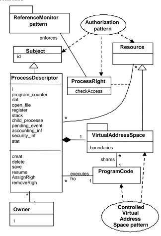
Figure 2. Class diagram for Secure Process
