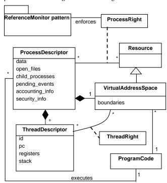
Figure 4. Class diagram for Secure Thread
