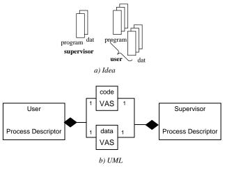
Figure 6. Two address spaces per process
