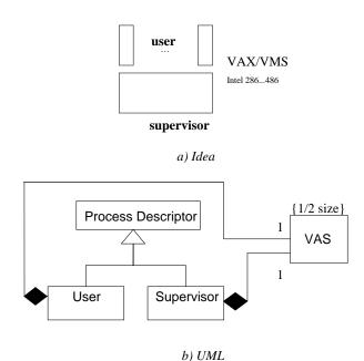
Figure 7. One address space per user process. All of them shared with the address space of the operating system.
