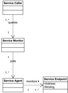
Figure 5. Service Monitor structure
