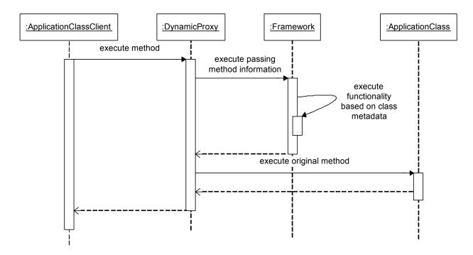
Fig. 11. Sequence of the proxy invoking the metadata-based framework.
