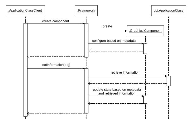
Fig. 15. Sequence of the interaction between the framework and graphical components.
