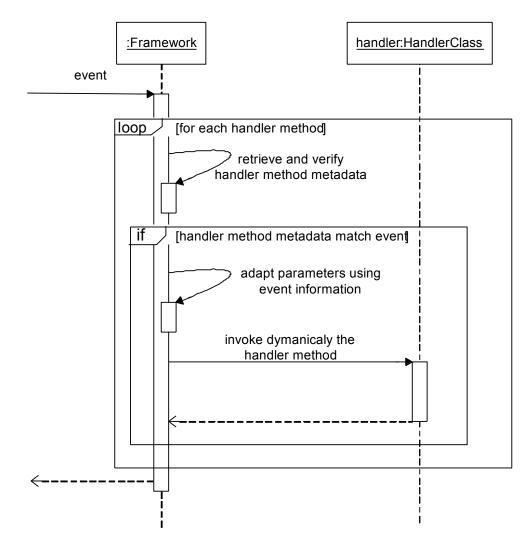
Fig. 7. Sequence of how the framework invoke the handler methods.
