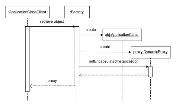
Fig. 10. Sequence of proxy creation using a factory.
