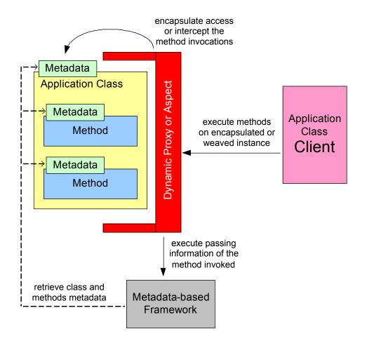
Fig. 9. The representation of Crosscutting Metadata Configuration.
