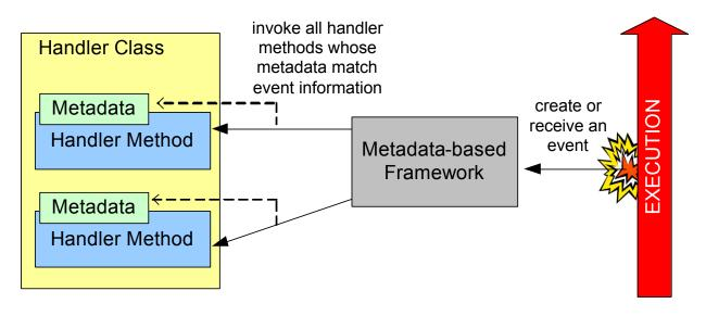
Fig. 6. Representation of the invocation of a Configured Handler Method.
