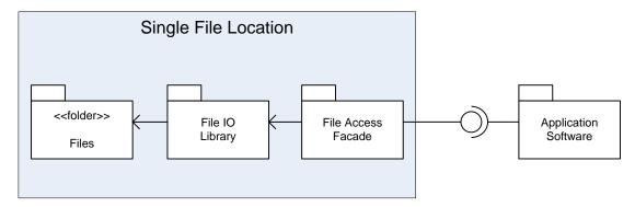
Fig. 4. Main solution structure for file access using SINGLE FILE LOCATION
