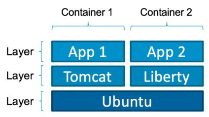
Fig. 1. Layers in Docker. This diagram shows how Layers in the docker filesystem are shared across containers.
