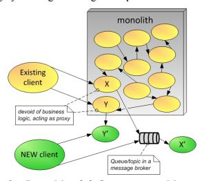
Figure 9—Proxy Monolith Components to Microservices
