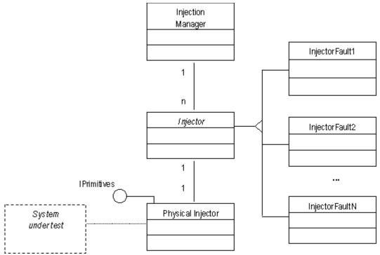
Fig. 2: "Injector" design pattern structure.
