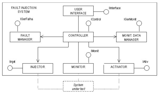
Fig. 1: "Fault Injector" architectural pattern structure.
