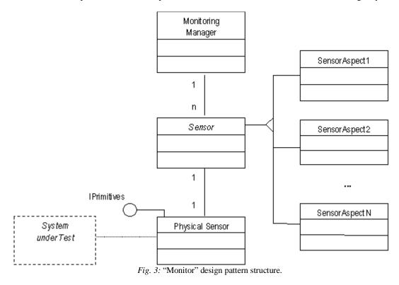
The interface *IPrimitives* designates the set of primitive operations that communicates with the target system.
