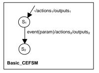
Figure 1. Basic CEFSM and its State Transition Diagram
