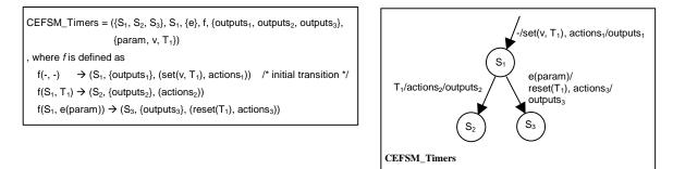
Figure 4. CEFSM with Timers and its State Transition Diagram
