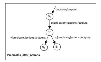
Figure 3. State Transition Diagram of CEFSM with Predicates after Actions
