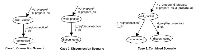
Figure 19. Packet Handling CEFSM using Source Merge
