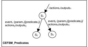
Figure 2. CEFSM with Predicates and its State Transition Diagram
