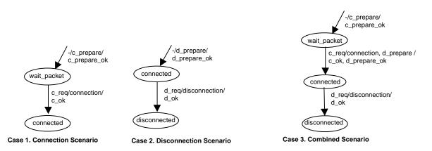
Figure 20. Packet Handling CEFSM using Sequential Merge
