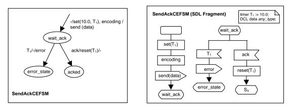
Figure 12. Example of Confirmed Data Transfer with a Timer
