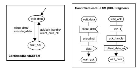
Figure 21. Confirmed Data Transfer using Mutual Merge
