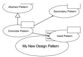
At the head of each pattern, we summarize the following description by using the standard UML representation for design patterns: the parameterized collaboration. Such a modeling element is represented as follows:
