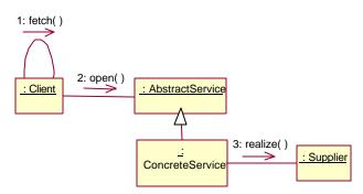
Figure 23: A collaboration diagram example.
