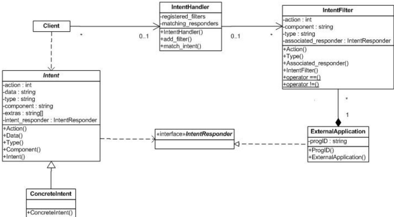
Figure 1. UML class diagram showing the structure. Abstract classes are omitted for brevity
