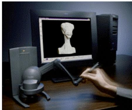
This image shows how a special input device, called The Phantom, is used in a 3D modelling application. This resembles how a sculptor would create a statue in the real world. The phantom has many degrees of freedom combined with haptic feedback so that the sculptor can actually feel the surface of the statue that is being designed.
