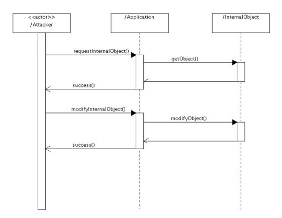
Figure 6. Sequence Diagram for the use case Compromise an Application with IDOR
