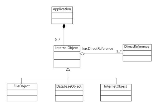
Figure 5. Class Diagram of the Insecure Direct Object Reference Threat Pattern
