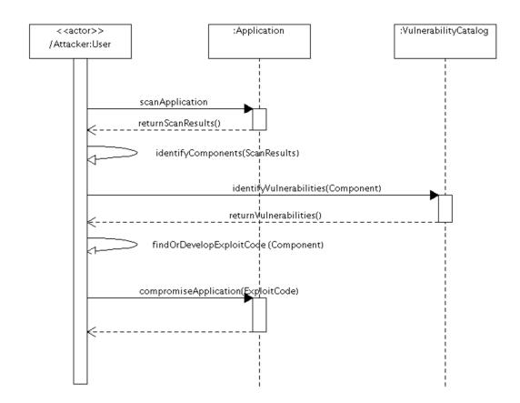
Figure 3. Sequence Diagram for the use case Compromise an Application using Vulnerable Components
