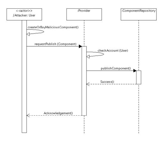
Figure 2. Sequence Diagram for the use case Publish a Malicious Component
