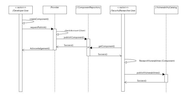
Figure 3. Sequence Diagram for the use case Unknowingly Publish a Vulnerable Component
