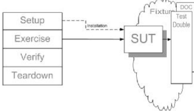
Sometimes it is just plain hard to test the [SUT](#) because it depends on other components that cannot be used in the test environment. This could be because they aren't available, they will not return the results needed for the test or because executing them would have undesirable side effects.
