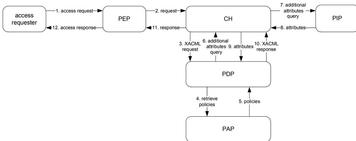
Figure 1: Overview of the data flow in the XACML authorization system (from [XAC04])
