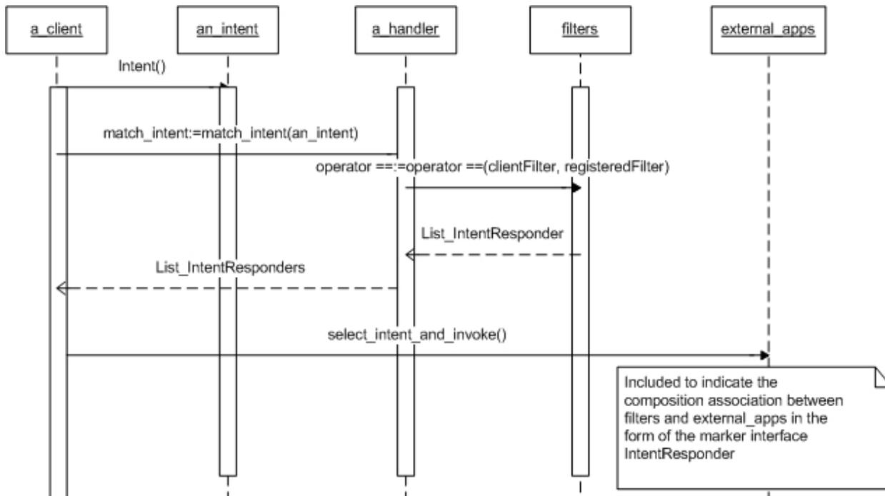
Figure 2. Sequence diagram showing the messaging involved from intent creation to resolution
