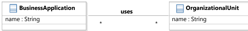
Figure 10: Information model fragment for variant of I-Pattern Business Application and Organizational Unit Relationship based on the uses variant
