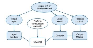
Fig. 2. Property-part diagram for the input-output system with an end-to-end check. As a consequence of the end-to-end check, the requirement no longer depends on the channel performing the computation correctly.
