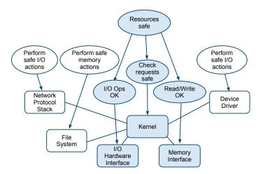
Fig. 8. Property-part diagram for a microkernel-based OS.
