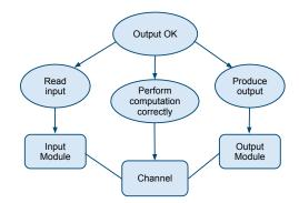
Fig. 1. Property-part diagram for an input-output system. A box represents a part, a circle a property, an arrowed edge a dependency of a property on a part or another property, and a straight edge an interaction between two parts.
