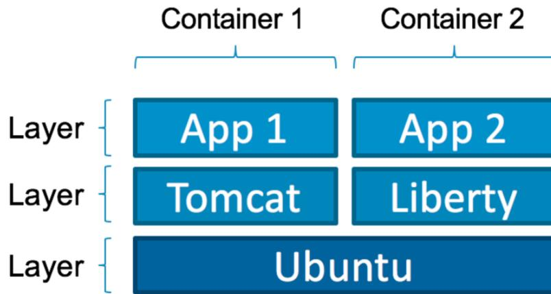
Fig. 1. Layers in Docker. This diagram shows how Layers in the docker filesystem are shared across containers.
