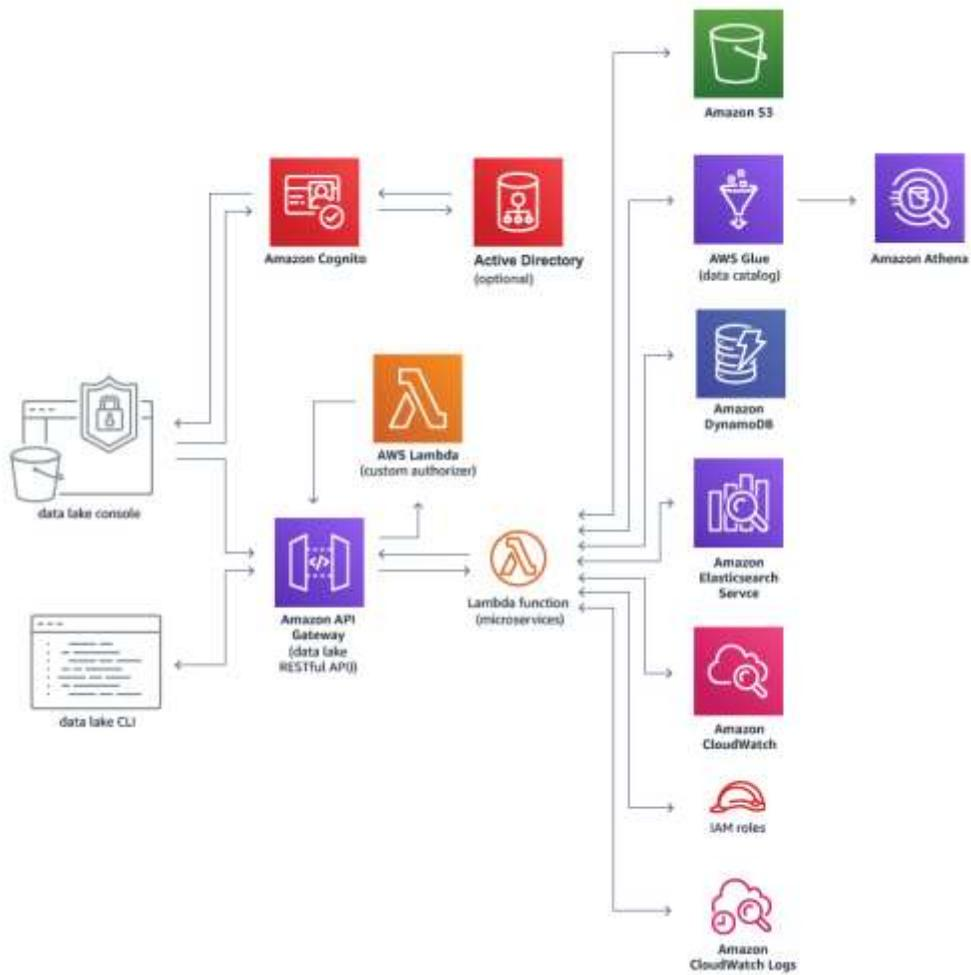
**Figure 4: Data Lake architecture in AWS [2].**
