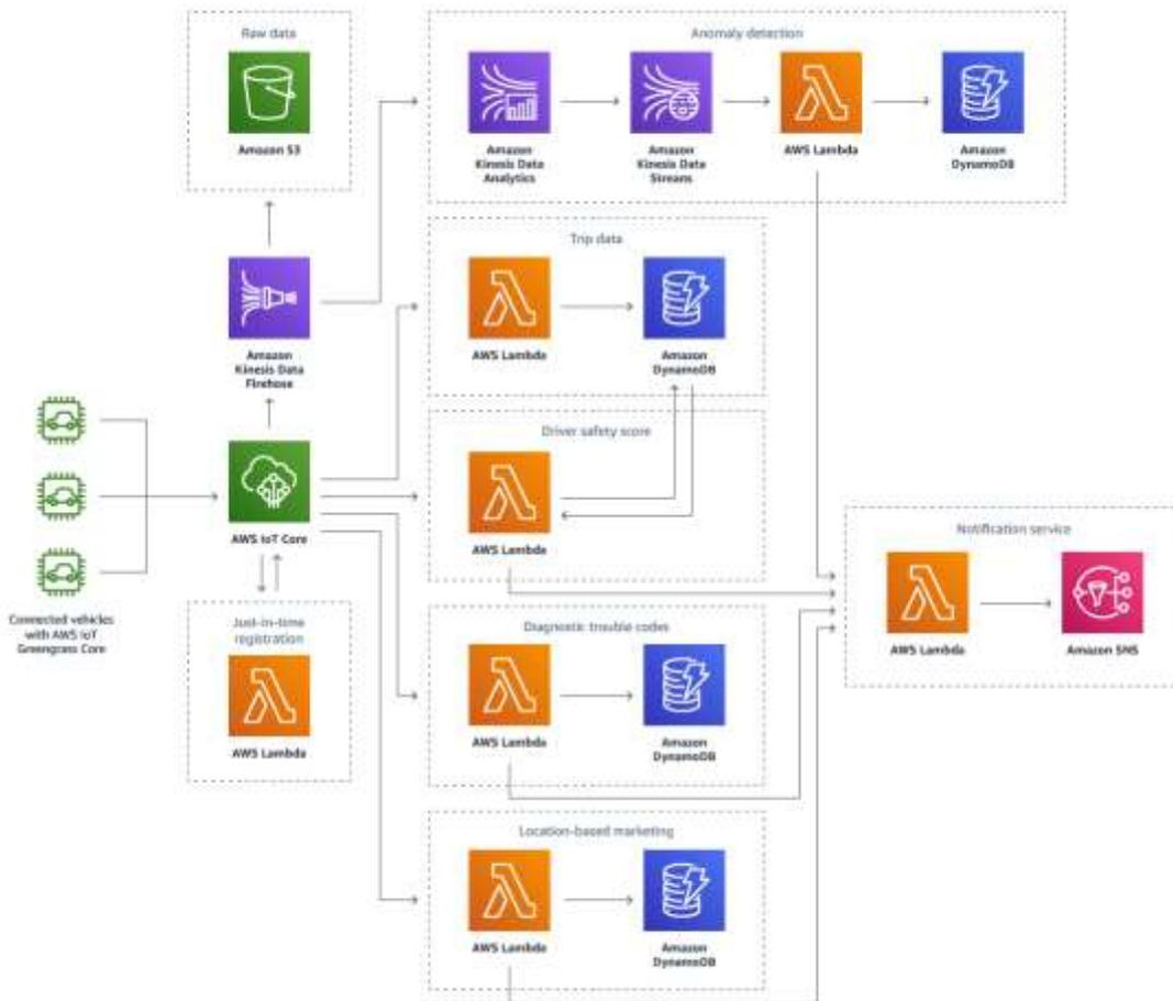
**Figure 6: Architecture of a connected vehicle in AWS [2].**
