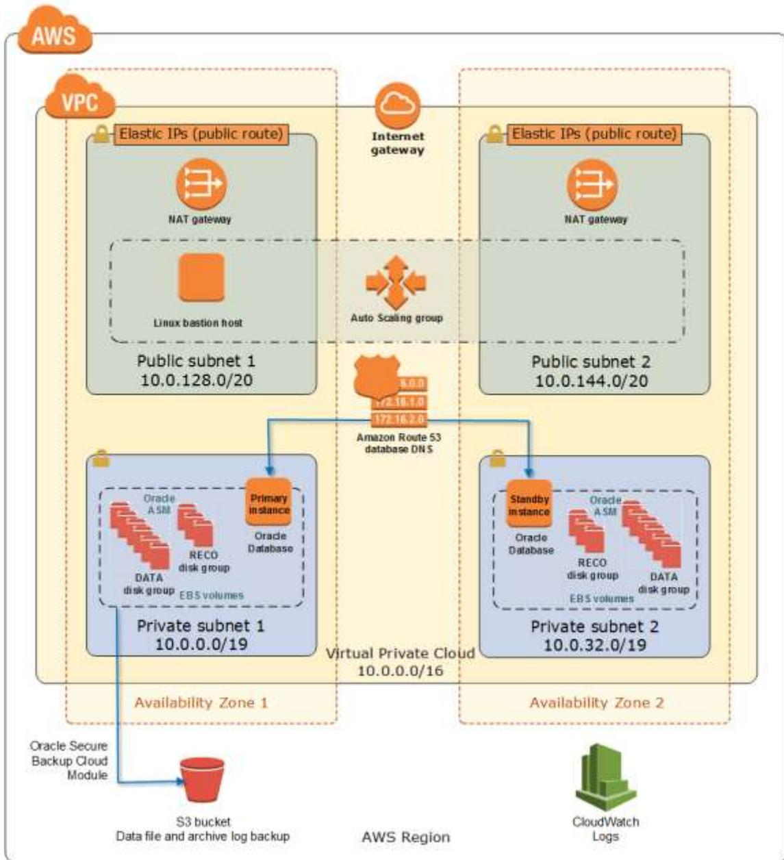
Figure 5: Architecture of a database system in AWS [2].
