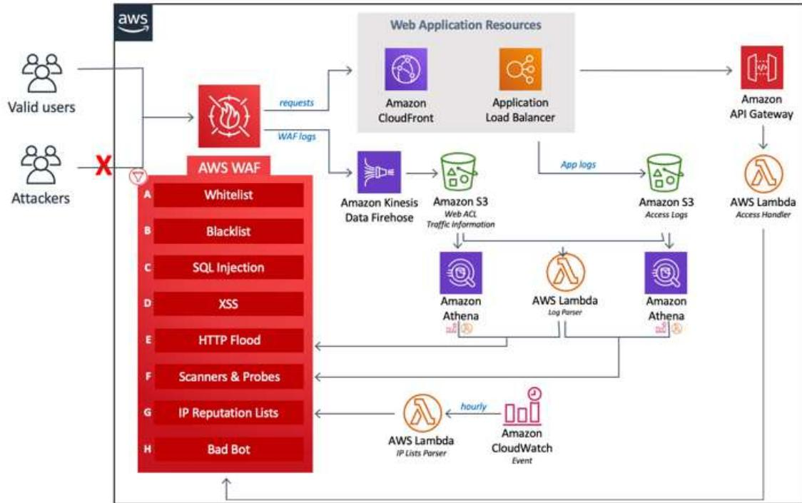
Figure 7: Architecture of a security front end in AWS [2].
