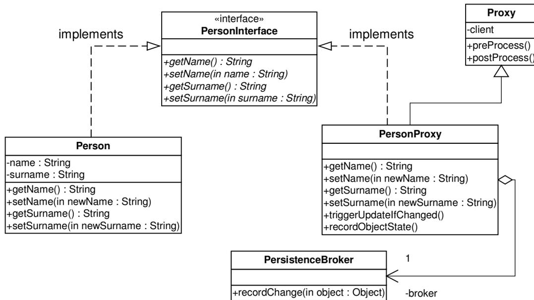
As in the second variation, the interface `PersonInterface` is used to connect the application layer (class `Person`) with the interception layer (abstract class `Proxy` and concrete class `PersonProxy`). The class `PersistenceBroker` is part of the framework layer.
