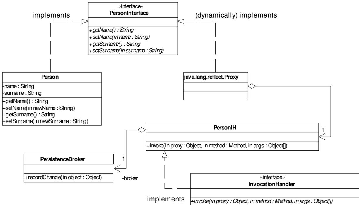
In this variation the interface `PersonInterface` is the key to connect the application layer (class `Person`) with the interception layer (class `Proxy`); the broker is part of the framework layer.
