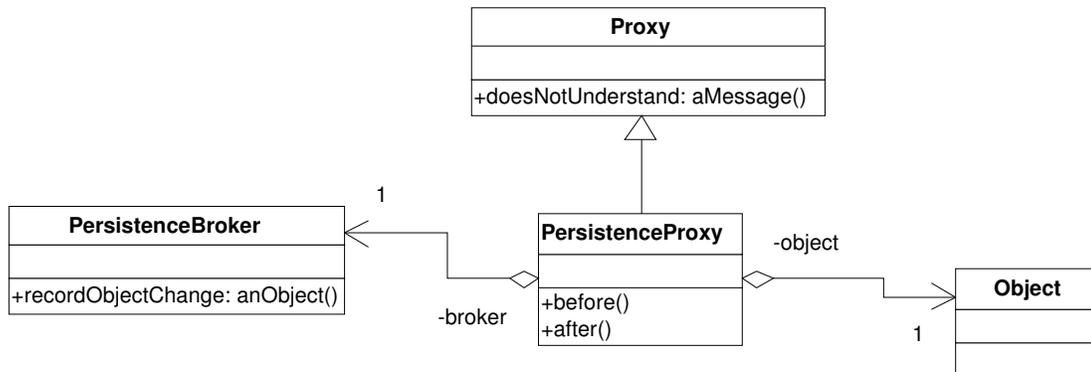
In this pattern the classes `Proxy` and `PersistenceProxy` would be placed in the interception layer, the class `PersistenceBroker` would be placed in the framework layer and the proxy's subject in the application layer.
