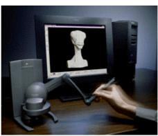
This image shows how a special input device, called The Phantom, is used in a 3D modelling application. This resembles how a sculptor would create a statue in the real world. The phantom has many degrees of freedom combined with haptic feedback so that the sculptor can actually feel the surface of the statue that is being designed.
